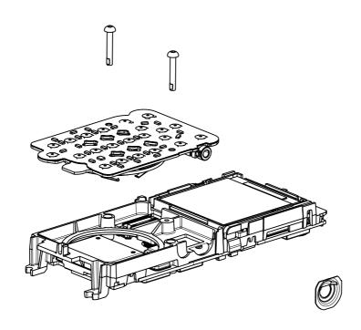
Figure 15 Keypad Board Removal and Installation
