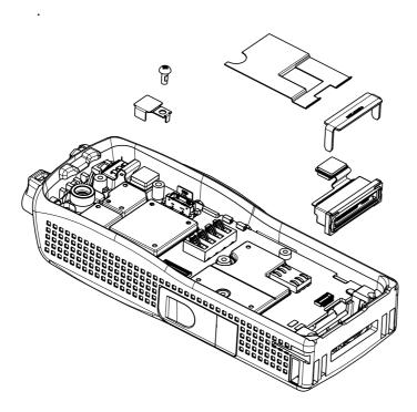
Figure 13 Removal and Installation of the Internal Assembly 1
