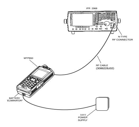
Figure 1 Typical Test Setup
