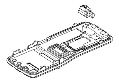
Figure 10 Vibrator Removal and Installation
