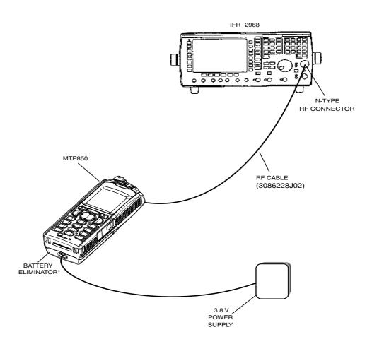
Figure 2 Typical Test Setup
