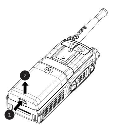
Figure 4 Battery Removal
