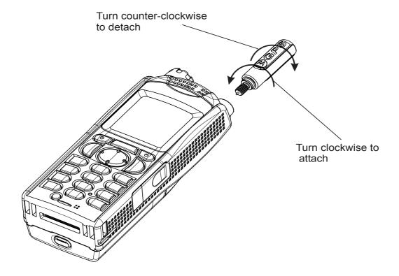
Figure 3 Antenna Removal and Installation
