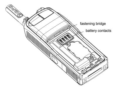
Figure 5 Location of Fastening Bridge & Battery Contacts
