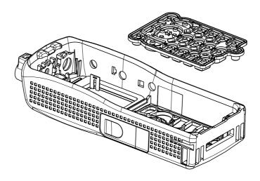
Figure 20 Keypad Removal and Installation
