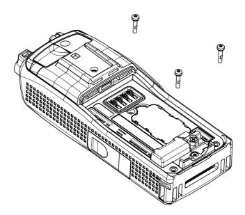
Figure 8 Back Housing Removal and Installation
