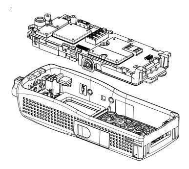
Figure 14 Removal and Installation of the Internal Assembly 2
