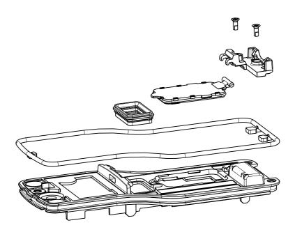
Figure 11 SIM Card Door Removal and Installation
