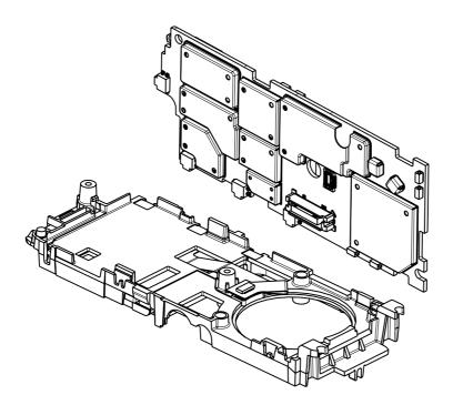
Figure 16 Main Board Removal and Installation
