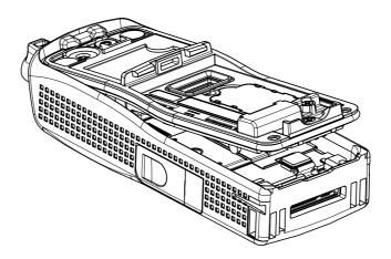
Figure 9 Back Housing Installation
