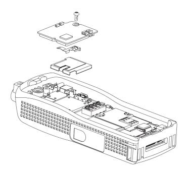
Figure 12 UCM Board Removal and Installation
